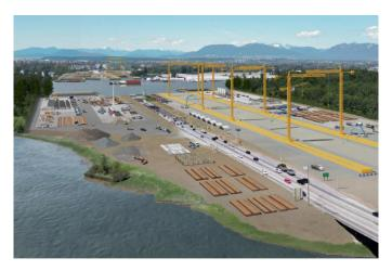
Next step is the construction of several 450-foot-long segments in a dry dock away from the bridge site.
